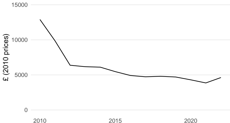
Figure 1: Mean total costs to install solar PV systems of 3 to 4 kW capacity.
