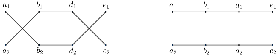
Figure 1: For any preference profile, the matching on the left is not stable; (a_1, b_1) is a blocking pair. The matching on the right is stable if a_1 and e_1 have client-lexicographic preferences. If a_1 has opponent-lexicographic preferences, (a_1, b_2) is a blocking pair.
